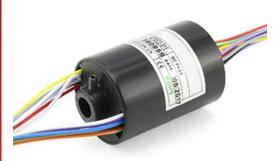
**CTH0317** series provides a 3mm through-bore for routing of hydraulic or pneumatic lines or hydraulic or pneumatic rotating shaft installation, and a compact 17mm outside diameter, features long life, fiber brush contact technology for ultimate performance in manychallenging applications.
